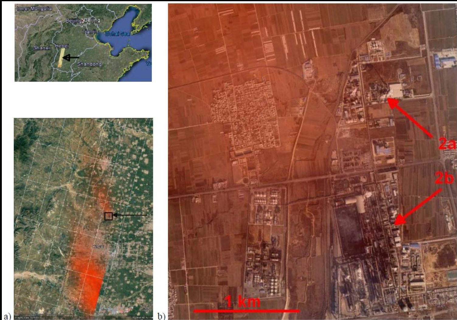
Figure 1. a) NO2 DSCD at 4:30UTC on September 29, 2016 retrieved by GSA algorithm. An arrow shows a square of a highly probable location of a source of NO2 pollution. b) The square from a) on an enlarged scale - some chemical industrial enterprise using coal, a possible source of the detected NO2 pollution. Maps of Google Earth for 12/2016 are used.
